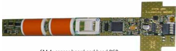
SM-1: sensor board and head PCB
